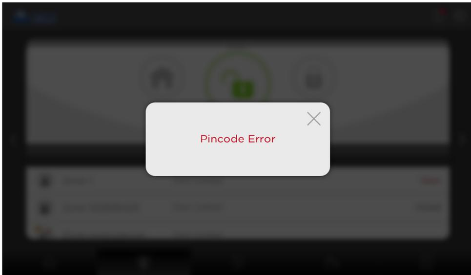
If the system has existing fault events when arming, the Panel will display fault messages and arming will be aborted.
