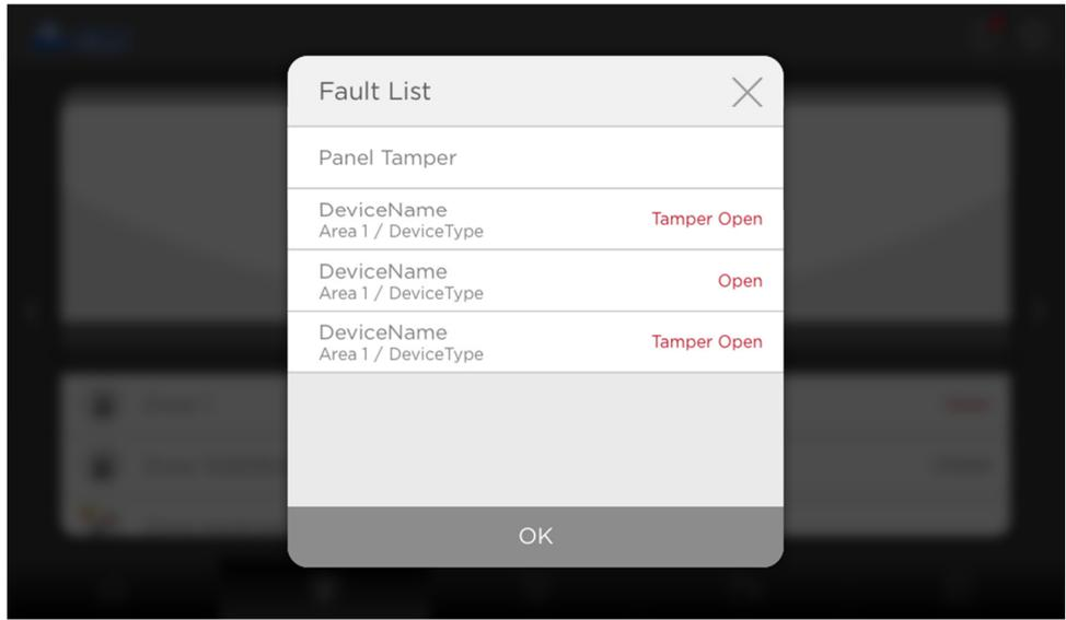
The system will prompt you to check all the faults, click bypass to acknowledge that you want to bypass faults displays and arm the system.
