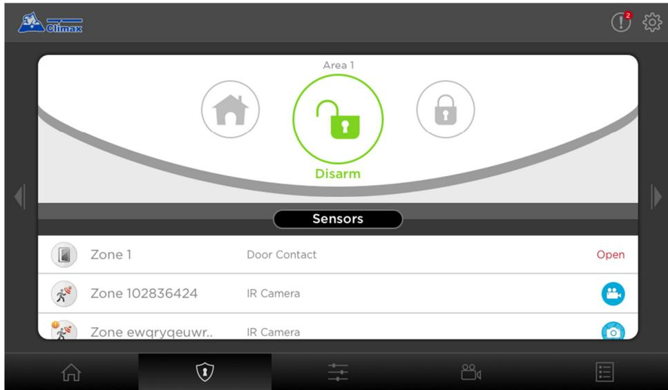
**System Mode:** The system mode is indicated by the 3 buttons at top. The current system mode will light up.
