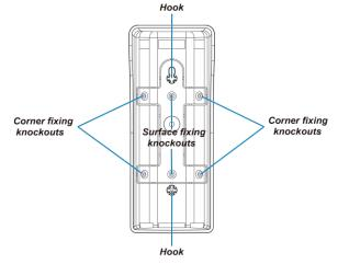
Two knockouts are for surface fixing and four knockouts are for corner fixing as shown in the picture.
