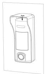
Please avoid mounting the PIR Camera on uneven sufaces. If mounting in a corner situation on uneven surfaces is still necessarey, you can attach the 4 adhesive foam spacers to the back of the mounting bracket to provide stress relaxation.
